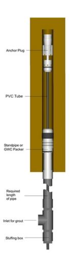
Anchor Plug is inserted in open rod line with PVC hose and stuffing box attached.
